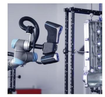
**Automated 3D system:** It can be paired with Scantech's automated 3D inspection system, enabling effortless deployment and intelligent control to conduct automated batch inspections.
