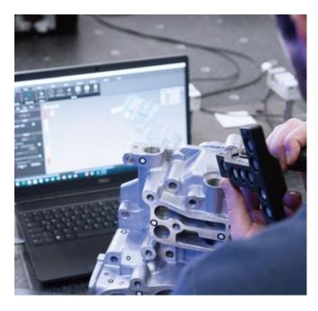
**Contact probing:** It can be paired with a portable CMM K-Probe to probe inaccessible areas and complex parts, offering comprehensive and precise 3D solutions.
